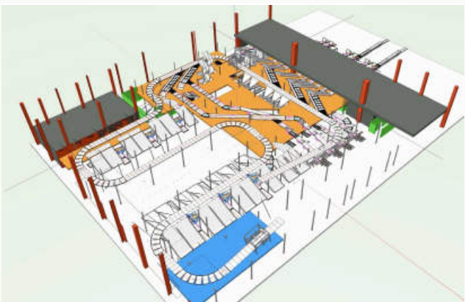
COORDINATION MODEL · SORTER WITHIN THE STRUCTURAL ENVELOPE · INSTALLED SORTING EQUIPMENT
