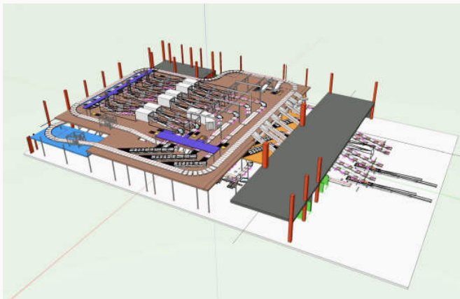
COORDINATION MODEL · SORTER WITHIN THE STRUCTURAL ENVELOPE · INSTALLED SORTING EQUIPMENT
